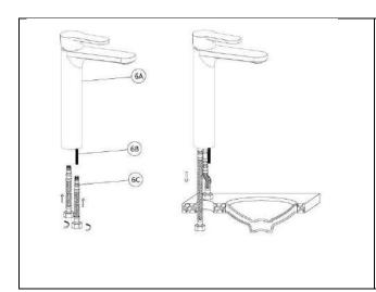
Install the two inlet hoses(6C) into the faucet(6A), these should only be hand tightened.
